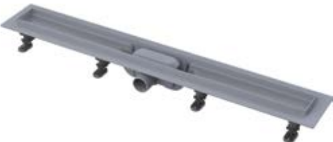
APZ8/9/10: 62 mm DN40 30 l/min
