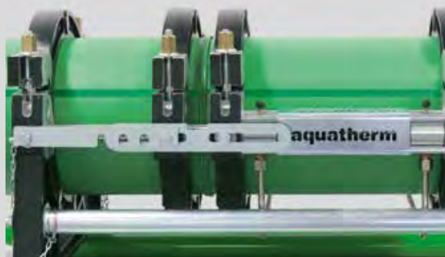
Join the pipes, cool down under pressure
