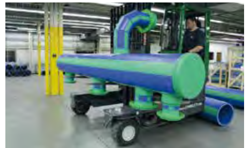
... aquatherm manifold construction.
