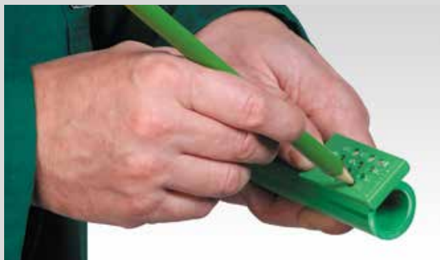
Marking of the welding depth
