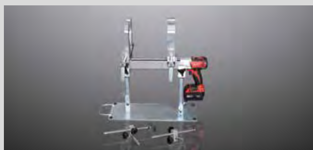
Electrical welding jig
